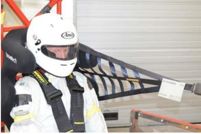
Figure 2: Photograph showing upper-strap inside the seat-side-head, shown with single-front-attachment design (internal view, but valid also for Dual-front-attachment)
